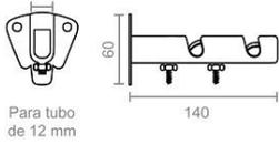
SOPORTE EN ACERO EXTENSIBLE Y DOBLE PARA BARRA DE 12 MM. MEDIDA 140X60 MM. ACABADO ZINCADO.
